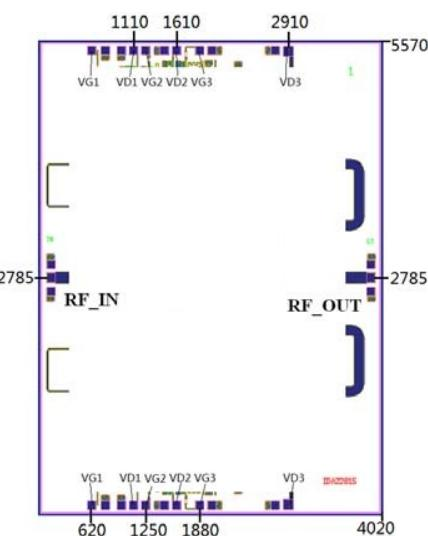
Note: The dimensions indicated in the figure are in micrometers (um); Input/output pressure point size 100×120μm<sup>2</sup>; The size of the bias pressure point is 100×100μm<sup>2</sup>.
