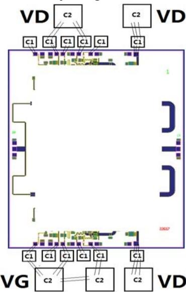
Note: Peripheral capacitors C1: 100pF, C2: 1000pF.
