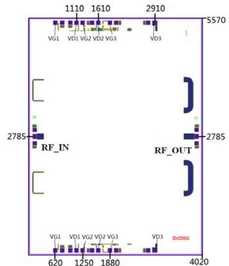
Note: The dimensions indicated in the figure are in micrometers (μm); Input/output pressure point size 100 × 120 μm<sup>2</sup>; The size of the bias pressure point is 100 × 100 μm<sup>2</sup>.
