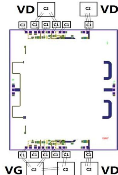
Note: Peripheral capacitor C1: 100pF, C2: 1000pF.
